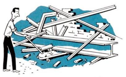
not practical for horizontal pulls. A gear-lifting device (Pul-Lift) has the advantage of no loose chain to get in the way. It takes little space and can be set up quickly.
