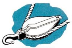
Some blocks can be opened from the side to allow easier threading of the rope. They are known as snatch blocks. Used properly, block and
