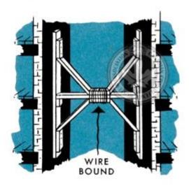
This shore uses a sound wall to support a sagging wall. It can be used for walls up to 25 feet apart. You'll see from the diagram that it is really only a series of four raking shores, each
