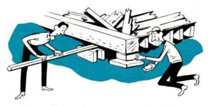
lever collapses, the victim may be injured even more. Always work from a secure position, keeping both feet on the ground.
