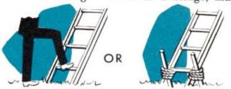
you've left plenty of overlap at each end. Place boards over the rungs to improve the footing.
