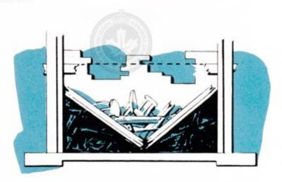
Sometimes the floor collapses in the middle, forming a "V" shaped pile of debris in the centre with voids on either side. Occasionally the centre of the floor holds up and both sides collapse, form-
