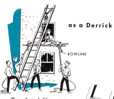
Two short ladders may be lashed together to make a longer one. Do it this way. Never tie on the rungs. Always the beams (sides.) Keep the knots on the under side.
