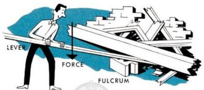
A lever is a device that gains power by sacrificing distance. It works like this . . . Any sturdy piece of wood or metal will make a lever. Any solid piece of masonry, etc., makes a good fulcrum. Learn to improvise.
