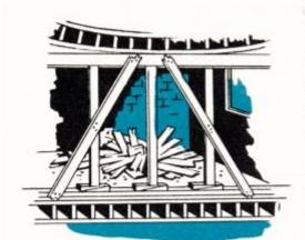
This type of shore bears a lot of weight. Therefore the sole piece should be very solidly placed. It should be as wide and as long as possible. Remember, the shorter the shore, the better it will carry a load.
