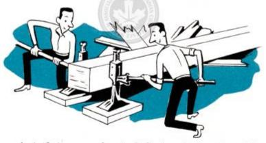
A jack is a mechanical device designed to lift heavy loads. You can use it in a more confined space than a lever. But it also needs care and practice to be used safely. You can practice using levers and jacks with equipment like this. Note: Before attempting to release a pinned-down victim, give him at least a pint of liquid. Always. If you fail to do this he may die.
