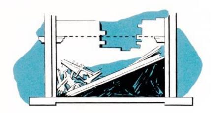
When floors drop on one side and hang to the wall on the other, a "lean-to" void is formed. They are often large and are relatively easy to reach.
